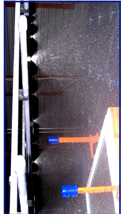
Water Recycling System (provides constant pressure filtered water during a water penetration test)
