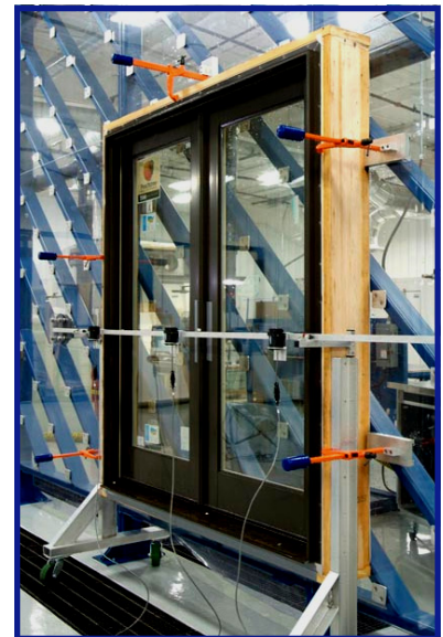
Deflection measurement equipment quickly mounted and ready for testing
